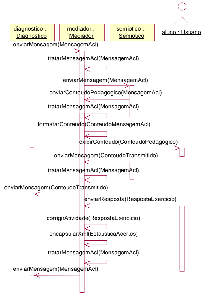
Figure 7.9: Sequence Diagram of Pedagogical Content Requisition and Exhibition by the Mediating Agent represented in UML (QUINTANS; PILATTI, 2002)
