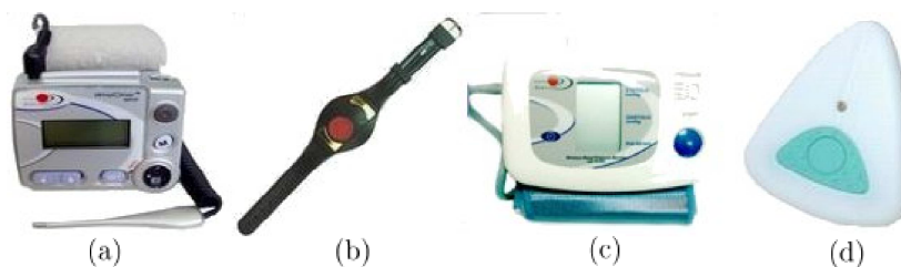
Figura 2.2: Sensores: (a) WristClinic TM , (b) MiniClinic Wrist-unit, (c) Wireless Blood Pressure Monitor BP100, (d) aLsis emergency unit da TelcoMed [62]
