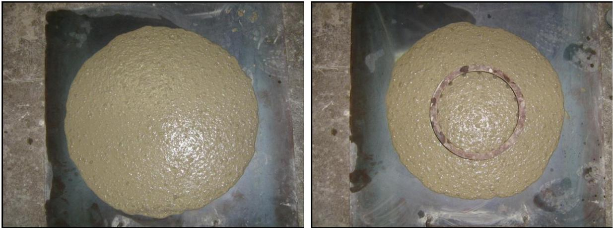
(a) *Slump flow*(b) *Slump flow com anel J*
