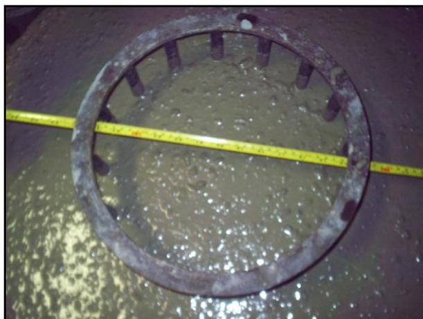
Figura 4.43 – Slump flow com anel J.
