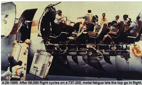
4-28-1988 After 89,090 flight cycles on a 737-200, metal fatigue lets the top go in flight.
