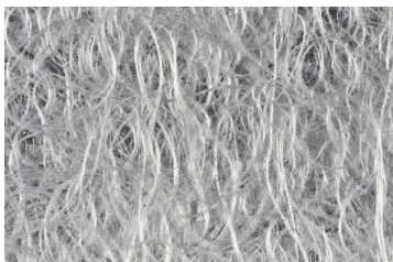
Figura 2.4 – Manta de fibras contínuas ( continuous strand mat )
