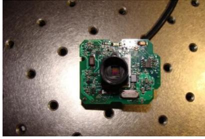
Figura 4.8 - Câmera CCD Webcan Logitech de 320x240 pixels
