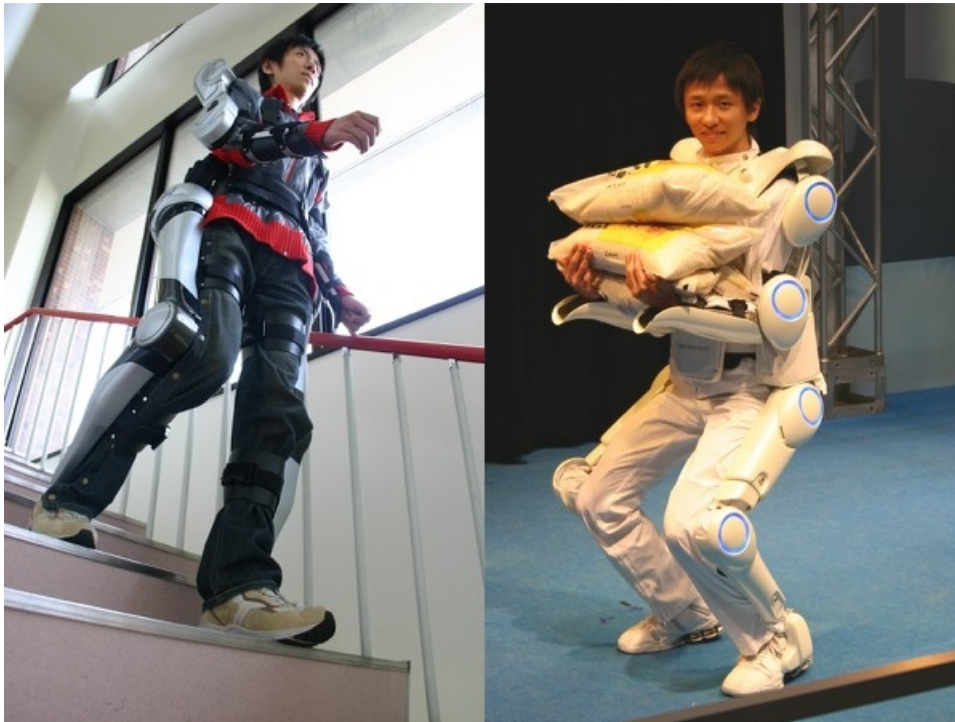
Figura 3.15: HAL - Hybrid Assistant Limb, [Sgarbi 2008].
