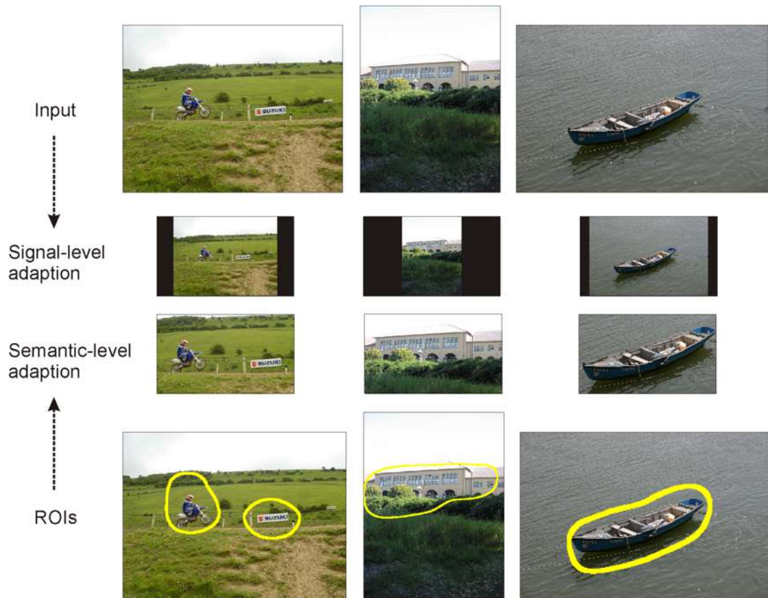
Figure 1.4: Example of the application of the proposed method for ROI extraction in a image adaptation scenario. Instead of being simply subsampled (signal-level adaptation), the original images can be semantically resized (semantic-level adaptation) to be displayed in a terminal with limited resolution and/or a particular aspect ratio.
