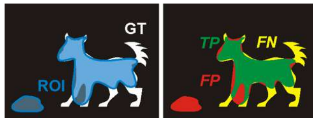
Figure 4.18: A synthetic example depicting a GT binary mask (white), the possible output of an ROI detector (blue) and the corresponding TP (green), FP (red) and FN (yellow) pixels.
