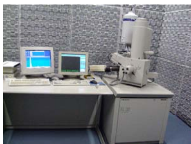
Figura 4- MEV, modelo XL 30 TMP, FEG, Philips, XL Series, com detector Oxford incaX-sight, Holanda, 97.
