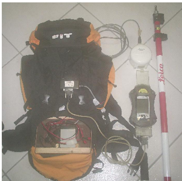
Figura 10 - Receptor DGPS (Differential global positioning system), Lab. de Geoprocessamento-UDESC/CAV, 2009 (Foto: Pablo G. Santos).
