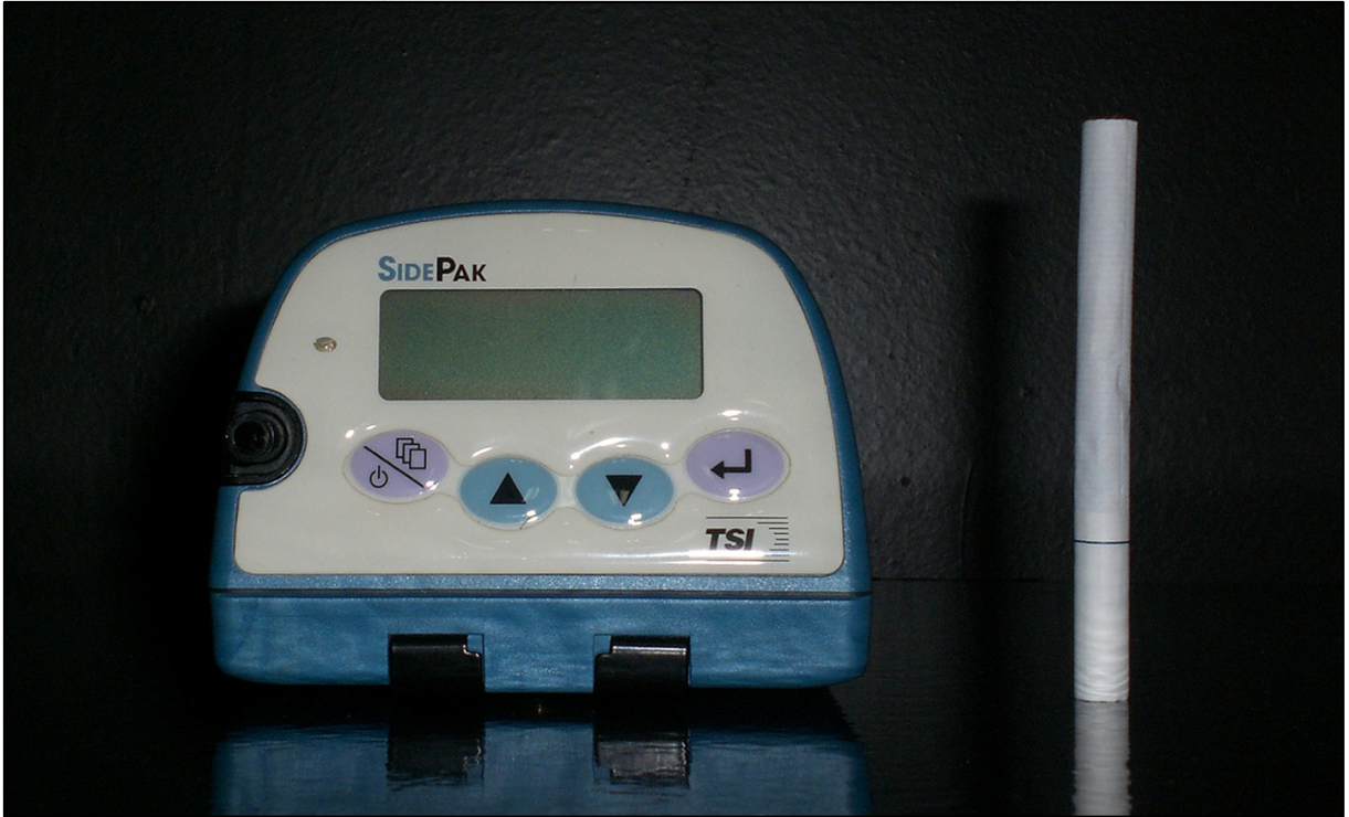
Figura 5.4 — Monitor de aerossol TSI SidePak AM510
