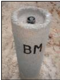
a) bench mark instalado
