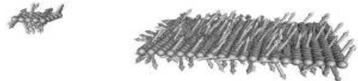
FIG. 2: Schematic view of our simulation arrangement. The tip is simulated as a 5 \times 5 rigid lattice of particles each carrying a spin \vec{S} . The surface is simulated as an arrangement of size 20 \times 20 . The tip is allowed to slid over the surface with initial velocity \vec{v} = v_0 \hat{x} . The arrows represent the spins directions.
