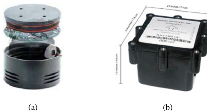
Figura 2.3. Magnetômetros de fluxo saturado modelos (a) Groundhog G-8, da Quixote Transportation Technologies e (b) VSN240-T, da Sensys Networks.
