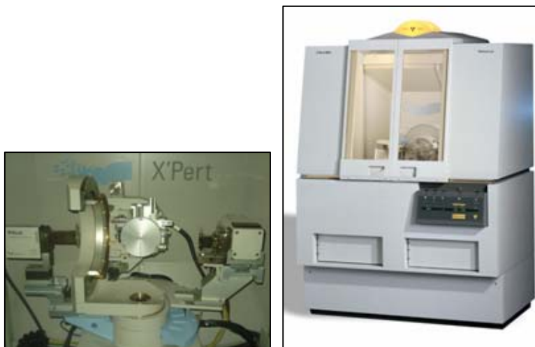
FIG. 3.21 Difratorômetro Panalytical modelo X'Pert Pro MRD
