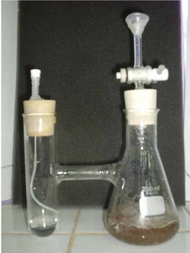
Figure 1: Biometer flask where it was make the microcosms experiment. In the Erlenmeyer like side it was inoculated the soil and biodiesel, the tube like side contain the NaOH solution that will uptake the CO<sub>2</sub> generate during respiration metabolism.
