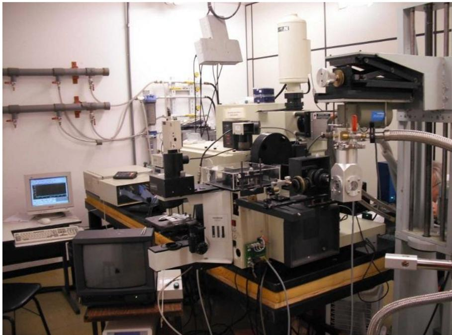
Figura 3.7 Espectrômetro Raman T64000 (fabricante Horiba Jobin Yvon).
