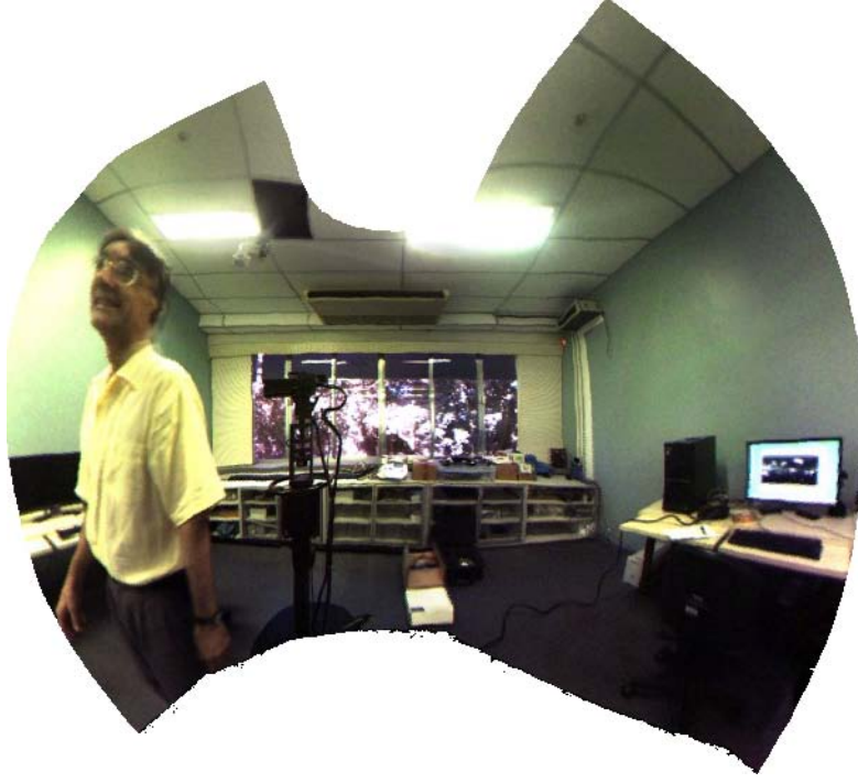
Figure 4.11: 16th frame for the video produced using only image energies. Due to the lines near the man, he is very curved in this frame. This fact demonstrates temporal incoherence, since he remains vertical in the input video.
