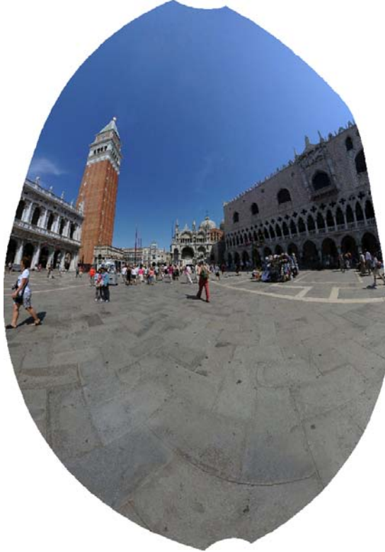
Figure 2.3: A result produced by the method if the user had only marked lines with no specified orientation. It seems that the tower is falling, for example. In order to avoid such problem, we give the user the possibility to specify the orientation of lines that she wants to be vertical or horizontal on the final result.
