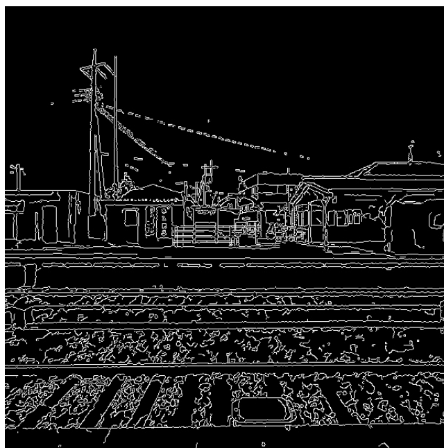
Figure B.16: Result of the edge detector applied after bilateral filtering. Some textures still remain and blurring more the image would blur too much the important lines.
