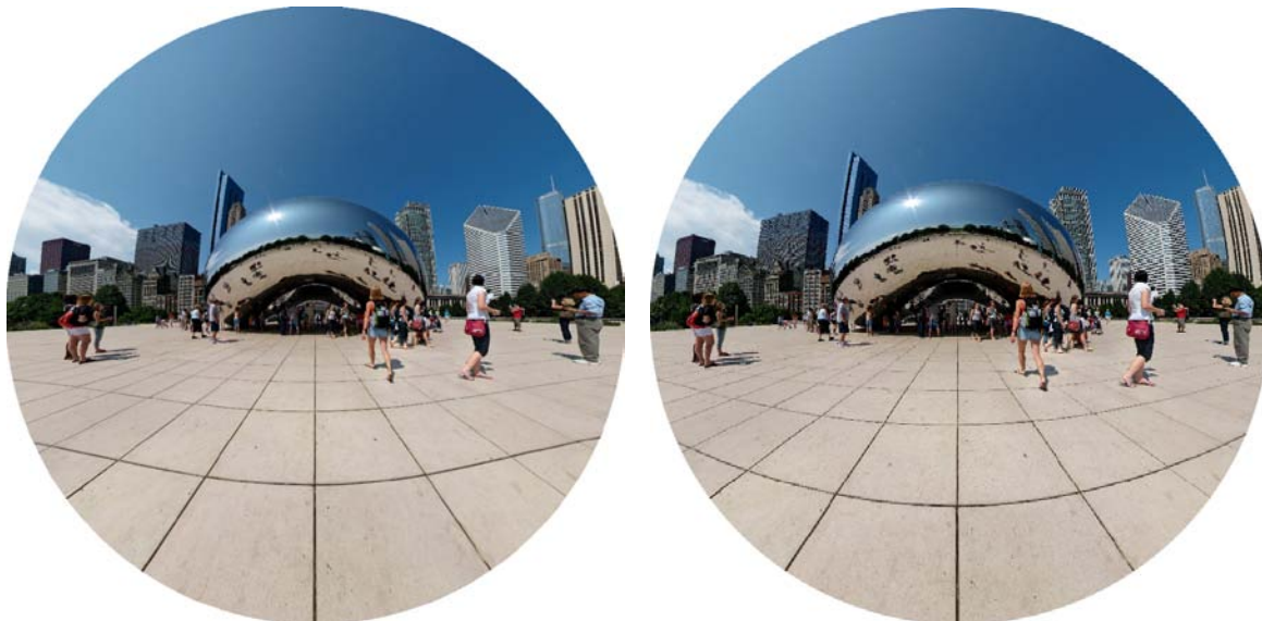
Figure 1.22: Both: 150 degree longitude/150 degree latitude. Left: \lambda = \frac{1}{2} ; Right: Perspective projection for K = \frac{1}{2} . Both have the same purpose of controlling the conformality and straight lines in the scene. Which one is better? The choices \lambda = \frac{1}{2} and K = \frac{1}{2} are arbitrary.
