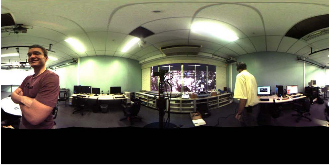
Figure 4.2: First frame of the video we use in this chapter. The camera we used does not capture the lower part of the entire field of view, i.e., the points with latitude near to -\frac{\pi}{2} .
