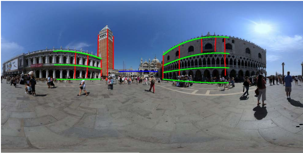
Figure 2.4: Equirectangular image with lines marked by the user. Red lines stands for vertical lines, blue for horizontal ones and green for general orientation ones.
