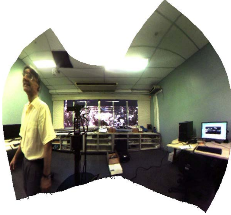
Figure 4.13: 16th frame for the video produced using image energies and object energy. Comparing to figure 4.11 the man is less curved, as expected. Now other problem arises: the projection for the entire scene changes too much to satisfy object constrains. One can observe, for example, that the borders of the projection from 8th frame to 16th frame change.
