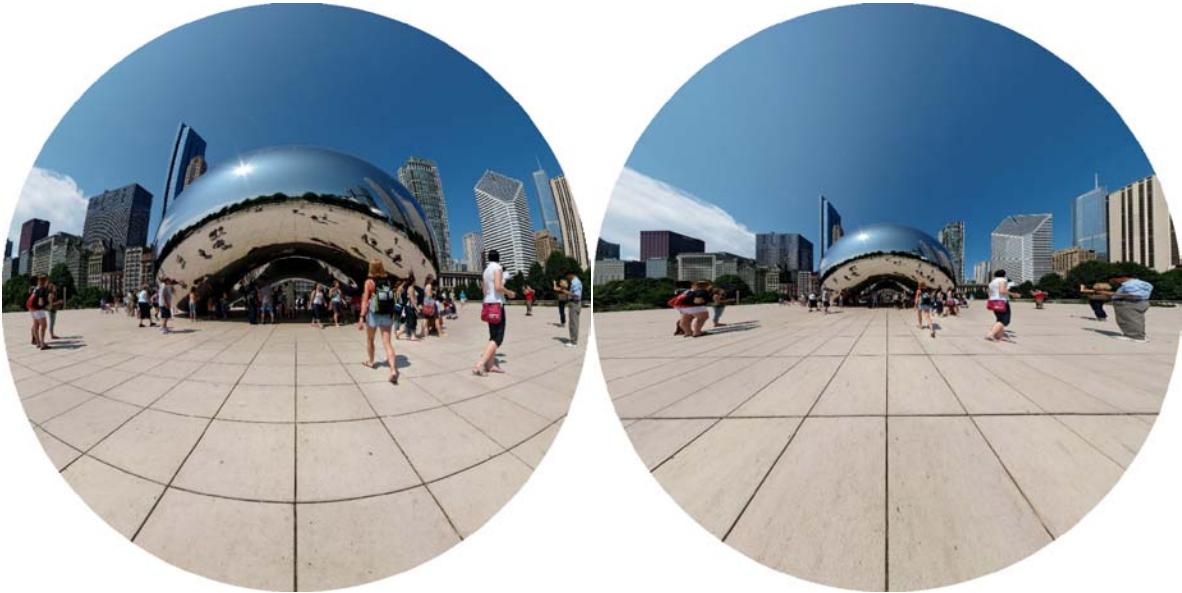
Figure 1.21: Both: 150 degree longitude/150 degree latitude. Left: \lambda = 0 (very similar to stereographic projection); Right: \lambda = 1 (perspective projection).
