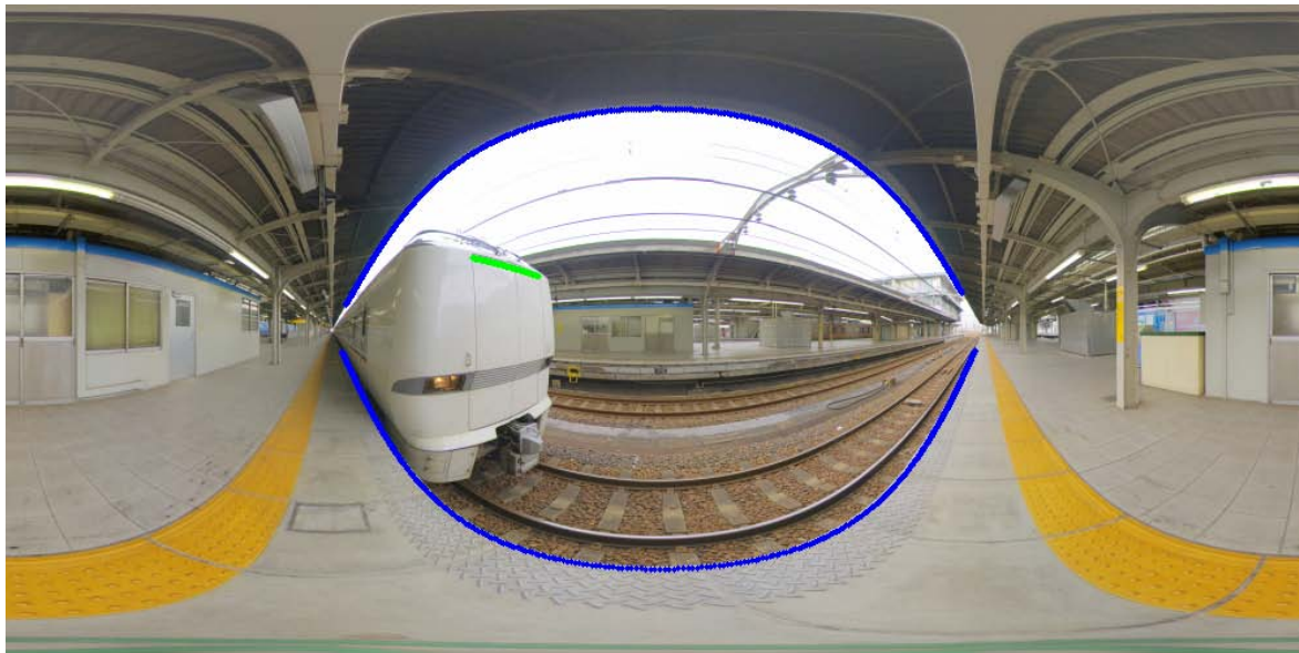
Figure 3.1: A scene with two horizontal lines covering near 180^\circ of the equirectangular image. Source image: “Express Shirasagi”, by Flickr user Vitroid.
