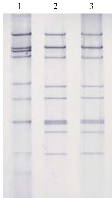
Figure 1. Electrophoretic migration pattern of RNAs, Brazilian P[6] genotype (P[6]-Gottfried-like and P[6]-M37-like) rotaviruses strains, finding in porcine stool samples, analyzed by electrophoresis in 7,5% polyacrylamide gel and visualized by staining with silver nitrate. Lane 1, P[6]-Gottfried-like genotype electropherotype "long"; lane 2 and 3, P[6]-M37-like genotype electropherotype "short".
