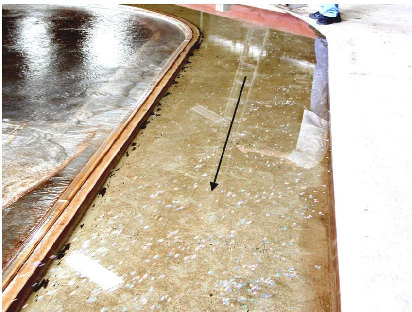
FIGURA 42 – VERTEDOIRO LIVRE – TRECHO FINAL – VAZÃO DE 720 m<sup>3</sup>/s
