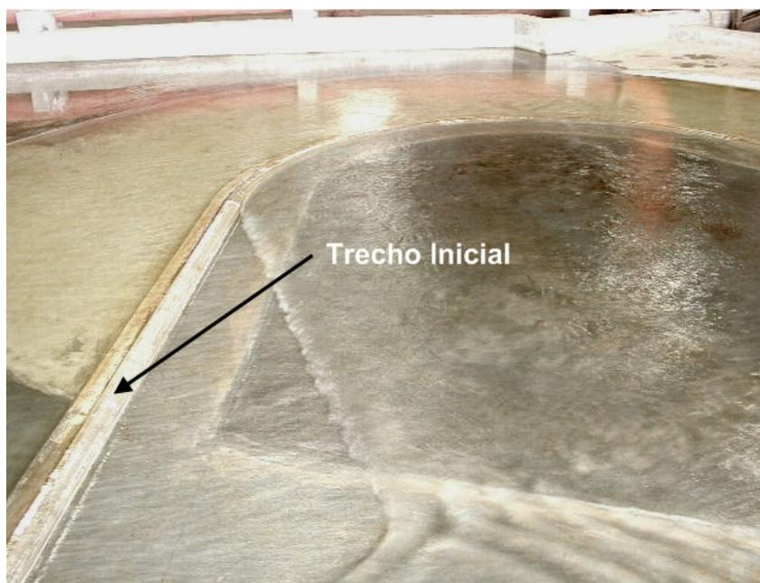
FIGURA 46 – VERTEDOIRO LIVRE – TRECHO INICIAL – VAZÃO DE 2880 m<sup>3</sup>/s
