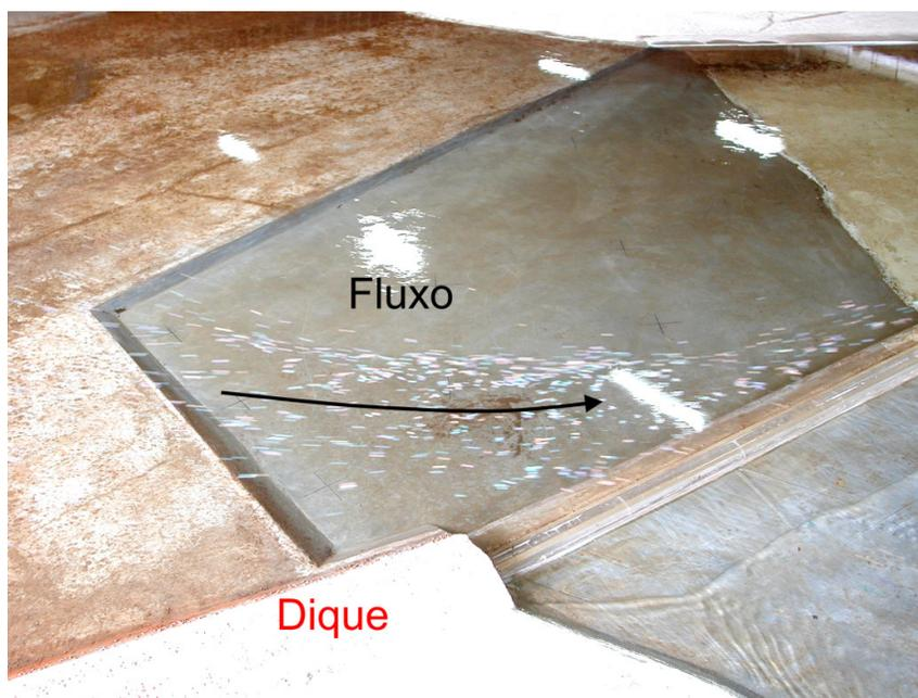
FIGURA 40 – VERTEDOURO LIVRE – TRECHO INICIAL – VAZÃO DE 720 m<sup>3</sup>/s
