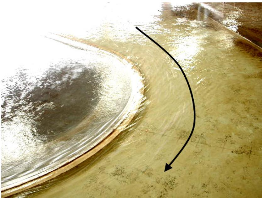
FIGURA 47 – VERTEDOURO LIVRE – TRECHO CURVO – VAZÃO DE 2880 m<sup>3</sup>/s
