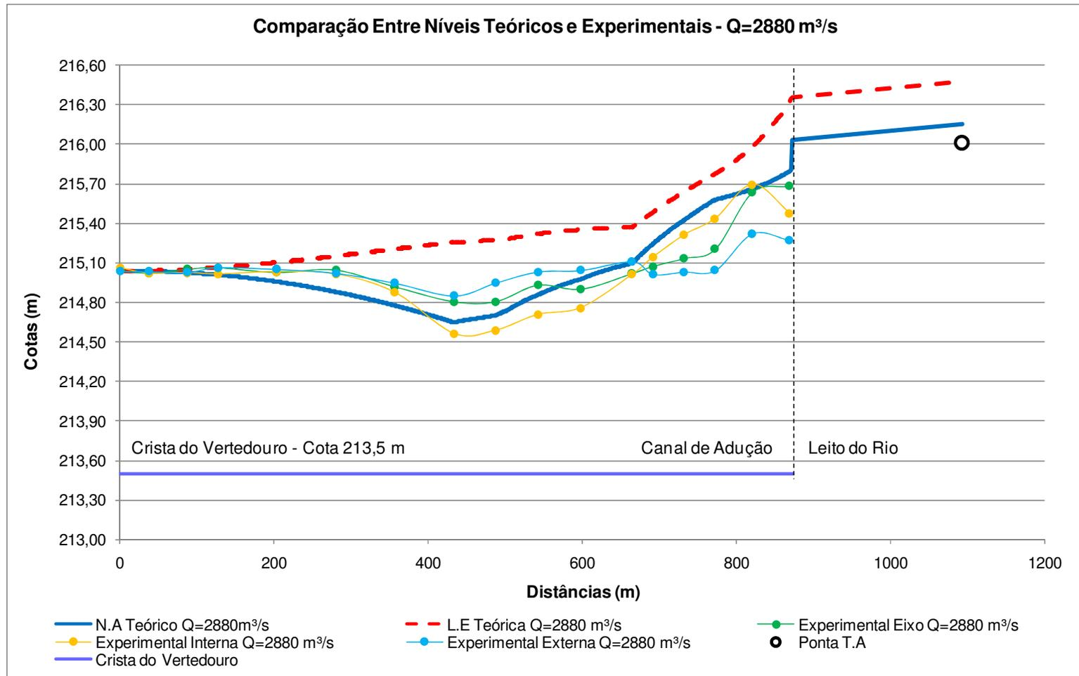
FIGURA 70 – COMPARAÇÃO ENTRE NÍVEIS TEÓRICOS E EXPERIMENTAIS – CÁLCULO SEQÜENCIAL – VAZÃO  $Q=2880 \text{ m}^3/\text{s}$
