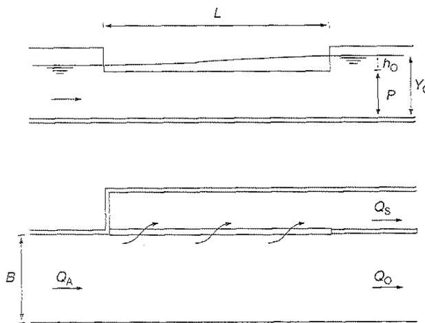
FIGURA 7 – VERTEDOURO LATERAL E CANAL LATERAL SOB ESCOAMENTO SUBCRÍTICO
