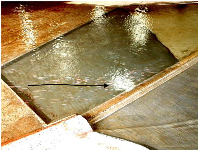
FIGURA 43 – VERTEDOURO LIVRE – TRECHO INICIAL – VAZÃO DE 1440 m<sup>3</sup>/s – COM VAZÃO TURBINADA
