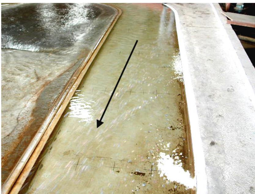
FIGURA 48 – VERTEDOURO LIVRE – TRECHO FINAL – VAZÃO DE 2880 m<sup>3</sup>/s
