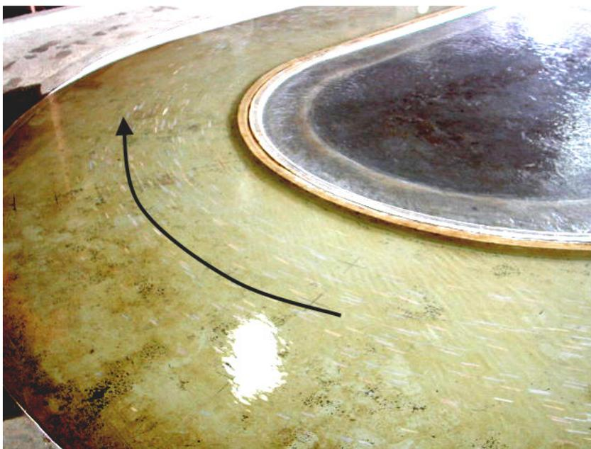
FIGURA 44 – VERTEDOURO LIVRE – TRECHO CURVO – VAZÃO DE 1440 m<sup>3</sup>/s – COM VAZÃO TURBINADA
