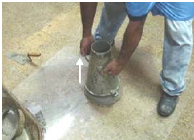
Figura 2.12 – Slump Test (LIMA, 2006)
