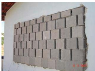
Figure 15: Photo of the block type 2 seated in the front separated 5 cm
