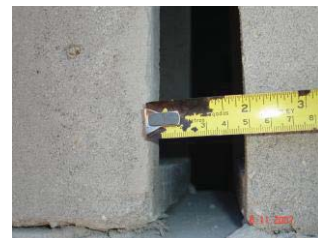
Figure 16: Photo of the block type 2 seated in the front separated 5 cm
