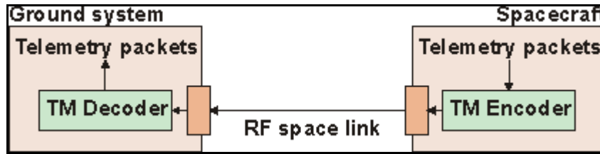
Figura 24: Spacecraft Packet Telemetry Overview
