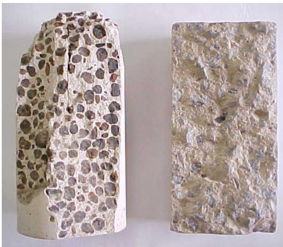
(a) Concreto leve
