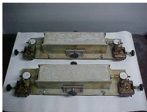
Figure 9. 1 – Autogenous shrinkage test
