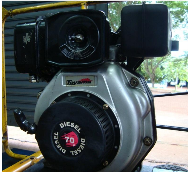
Figura 3.1 Motor Toyama T70f.
