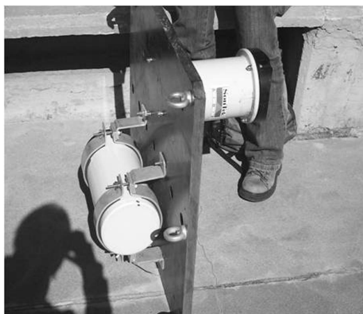
Figure 4. Details of the ADP (Sontek) equipment used for current measurement.
