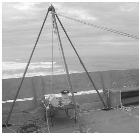
Figure 5. Tripod used to launch the ADP into the surf zone.
