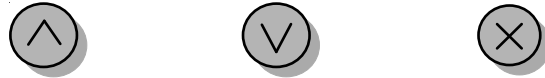
Figure 2.11 Rules used in EPCs. The first (from left to right) symbols an “AND rule”, the second symbols an “OR rule” and the third symbols an “EXCLUSIVE-OR rule”
