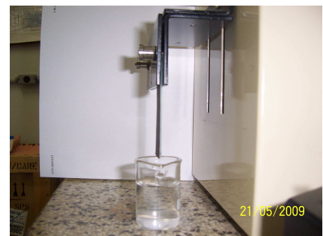
Figura 2: (1) Sistema dip-coating . (2) Forno. (3) dip-coating - Frontal. (4) dip-coating - Lateral.
