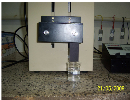
Figura 2: (1) Sistema dip-coating . (2) Forno. (3) dip-coating - Frontal. (4) dip-coating - Lateral.
