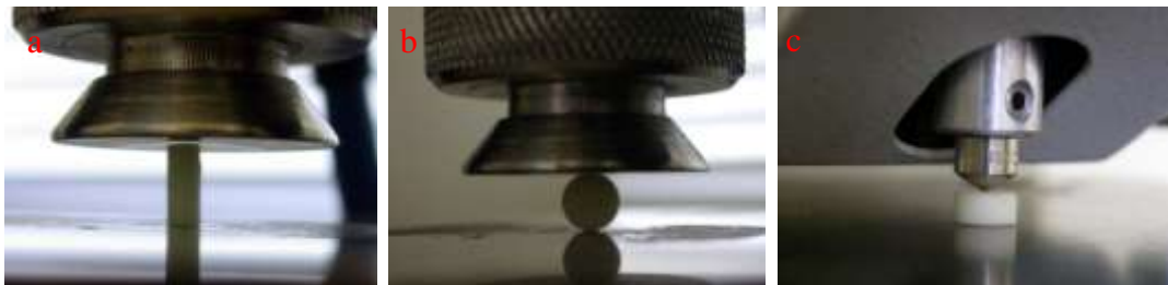
Figure 1. Mechanical tests in progress: Compressive strength (a); Diametral tensile strength; and (b) Microhardness (c).
