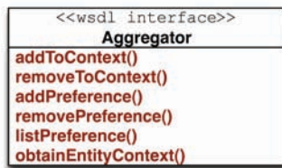
Figure 5.12: Aggregator service interface
