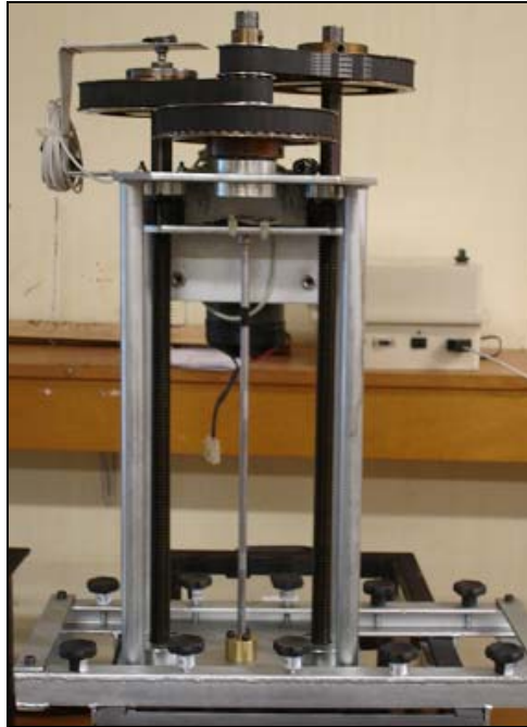
Figura 3.11: MCPT - Miniature Cone Penetration Test (Fonini, 2008).
