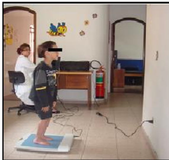
Figure 1: Assessment of static balance with Fusyo platform
