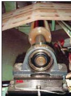
**FIGURA 2.13 – CÉLULA DE CARGA. (Cortesia: ABB)**
