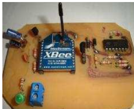
Figure 4. Diagram of the End Device Sensor (Filho and Dias, 2008).
