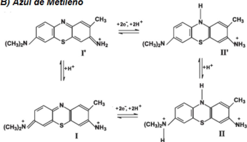
**FIGURA 17** – Influencia do pH na molécula do azul de meldola(A) e na molécula do azul de metileno(B). Figura adaptada da referencia *J. Braz. Chem. Soc.*, Cationic Dyes Immobilized on Cellulose Acetate Surface Modified with Titanium Dioxide: Factorial Design and an Application as Sensor for NADH, Vol. 18, No. 8, 1462-1472, 2007.
