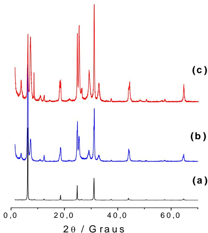
**FIGURA 13** – Difratogramas de Raios-X **Vs** (a), **V/Cu** (b) e **V/Co** (c).
