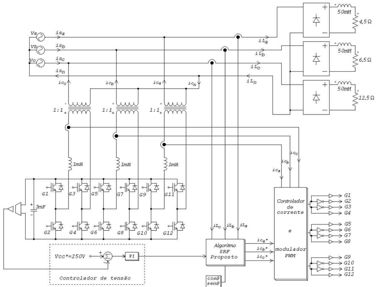
Fig. 5.9 - FAP trifásico topologia *Three Full-Bridge*
