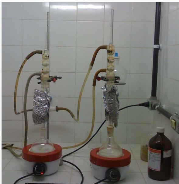
Figura 3.4: Extrator de soxhlet
