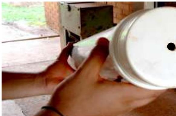
FIGURA 3 - DRENAGEM DAS COLUNAS DE SOLO MONTADAS
