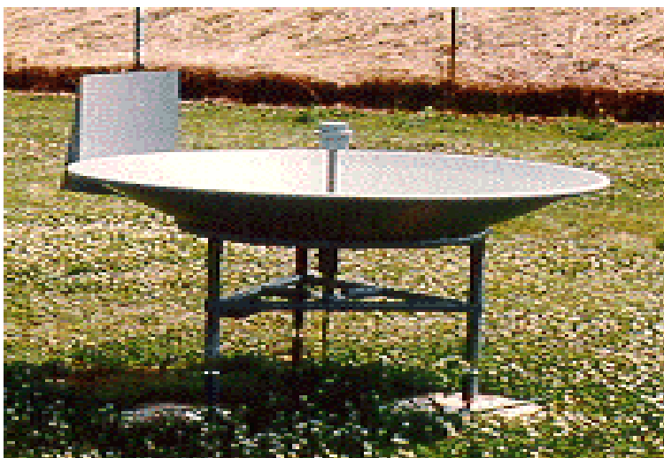
Figura 3.11: O SODAR (Fonte: http://www.jhu.edu/~dogee/mbp/research/lidar/main.htm ).
