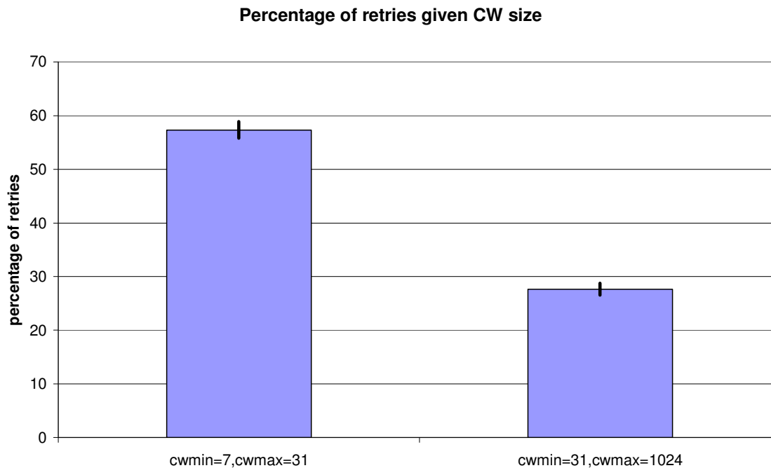
Figure 37 – The percentage of retries in icmp echo responses (with error bars) triggered by ten nodes pinging the multicast address (224.0.0.1).
