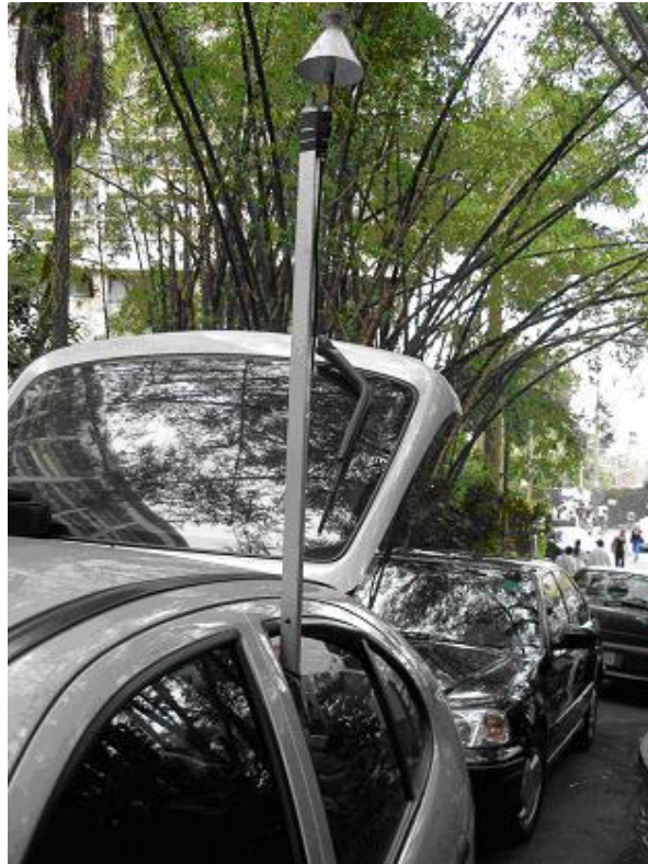
Fig 4.2 – Antena do receptor instalada.
