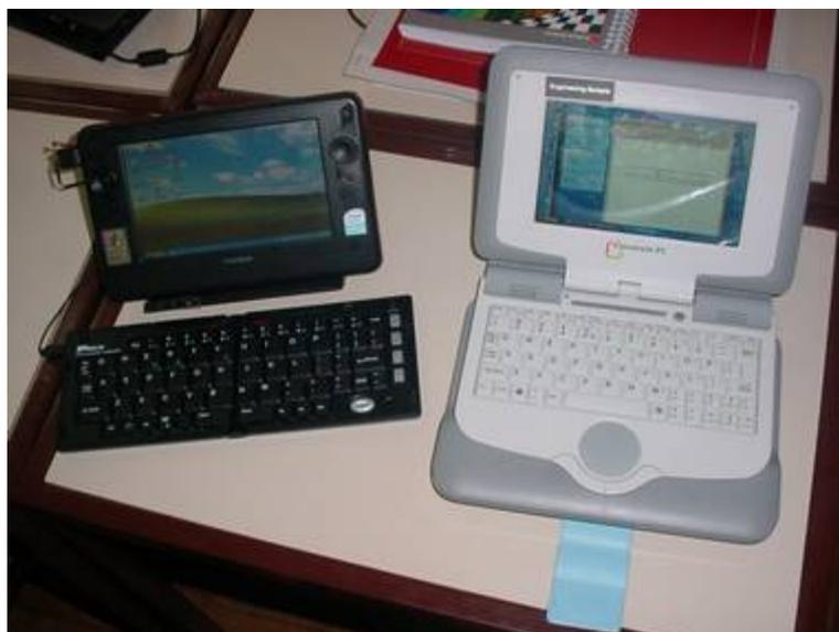
**Figura 06 – UMPC (*Ultra Mobile Portable Computer*) na esq. e CMCP (*Class Mate Portable Computer*) na dir.**
