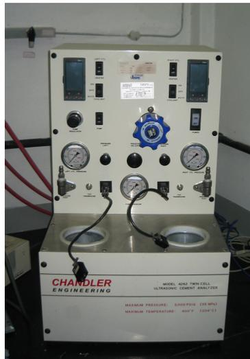
Figura 5.5. Equipamento *Ultrasonic Cement Analyzer* (UCA)
