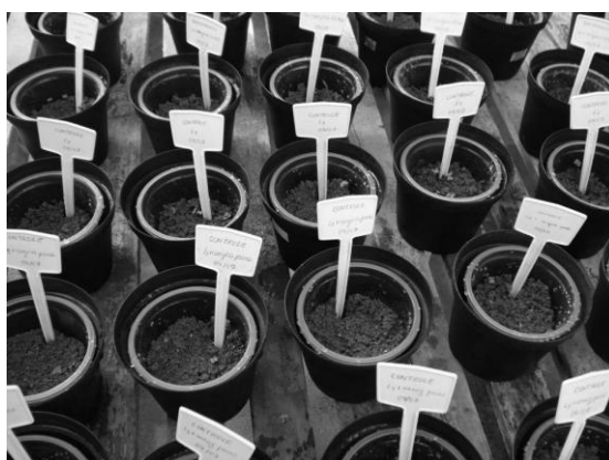
Fig. 2. Soil microcosm: 350 cm 3 transparent polypropylene pot containing 200 g of untreated soil, inside 500 cm 3 opaque plastic vase, under greenhouse conditions
