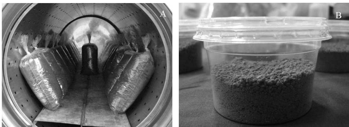
Fig. 2. (A) Soil pasteurization in autoclavate polyethylene bags; (B) Soil microcosm: 145 cm 3 transparent polypropylene pot containing 40 g of pasteurized soil.
