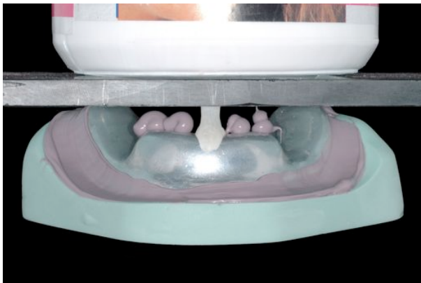
Fig 5 Standardized pressure of 1.25 kg.
