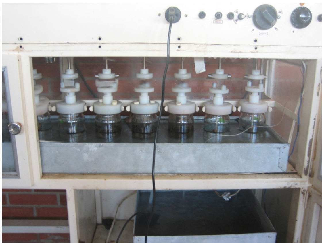
Figure 6. Apparatus utilized for enzymatic hydrolysis.
