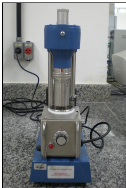
Figura 4.16 – Viscosímetro coaxial Chandler
