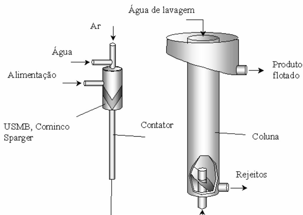
**Figura 22.** Coluna Contact Cell.
