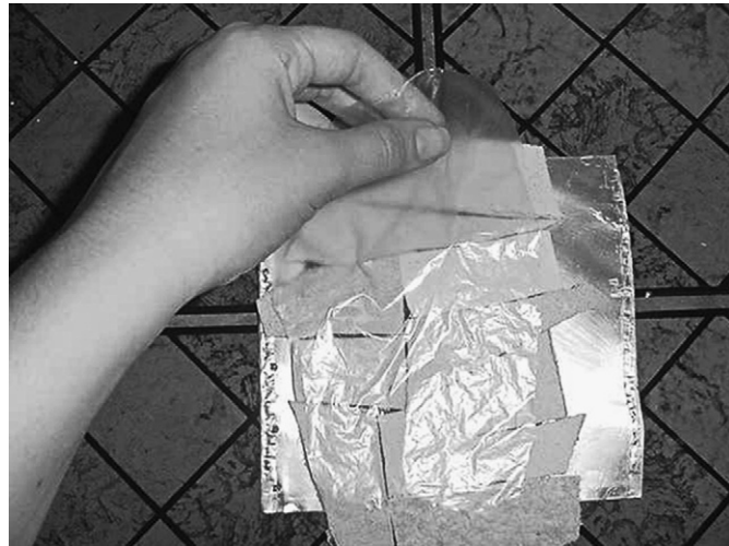
Fig. 7. Assembly of the hot melt second layer.
