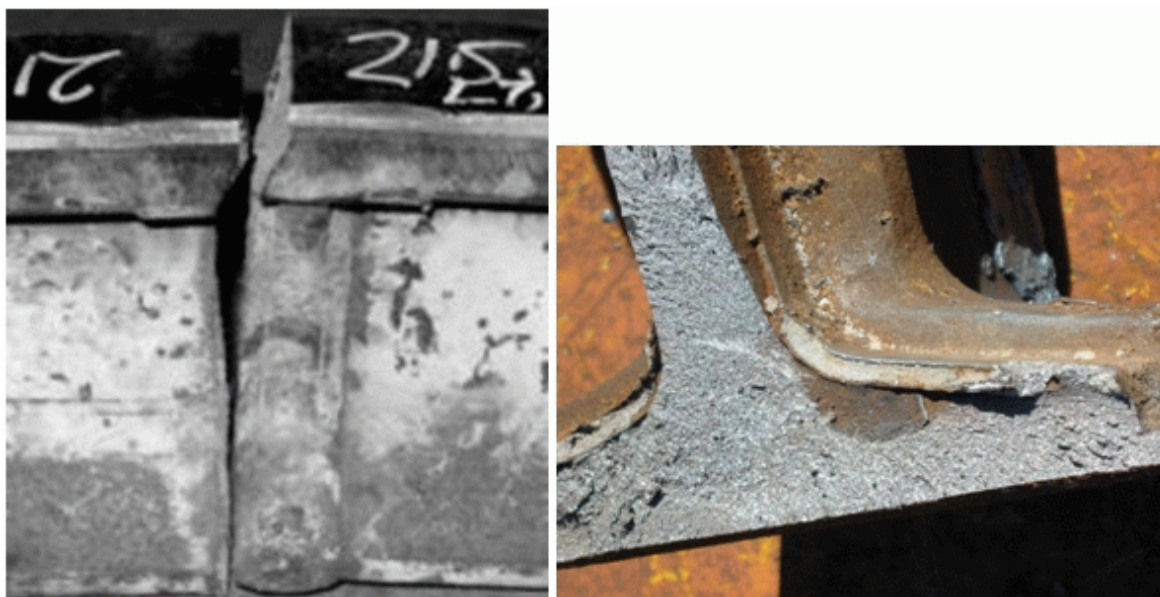
Figura 2.28 – Fratura Transversal (MUTTON, 2004) e (DUVEL, 2005).
